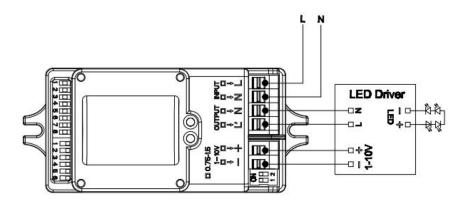
\*The sensor is designed for connect one load only. Connect more than one loads may damage the sensor.
