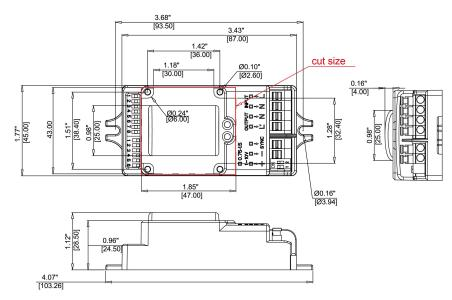
\*To aviod blocking microwave transmitting, please cut hole as image above to make sure microave antenna exposed froom any metal.
