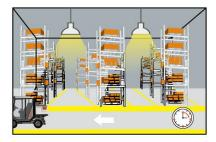
After elapse of hold time, the sensor dims the light at the present low light level if no motion is detected.
